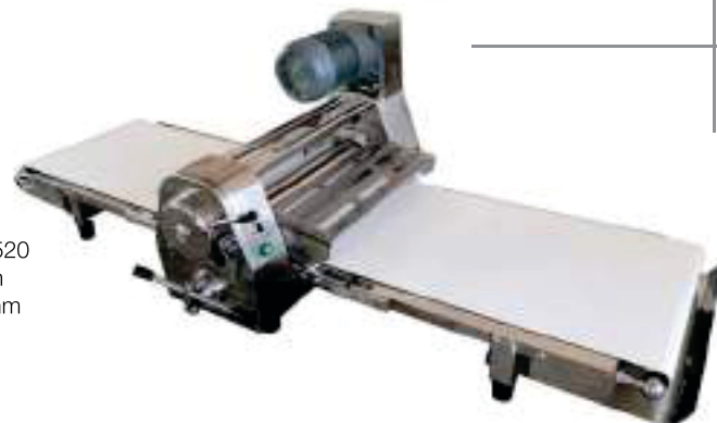
Pizza Sheeter, T40 Size: 370x565x715mm Power: 390W Short Roller: Ø25xØ45x300 Longe Roller: Ø48xØ25x422
